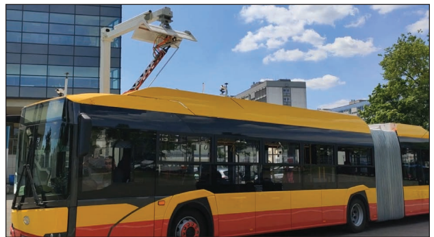
FIGURE 1 An Urbino 18 articulated urban bus, manufactured by SBC, docked with a pantograph at a mockup charging station.
